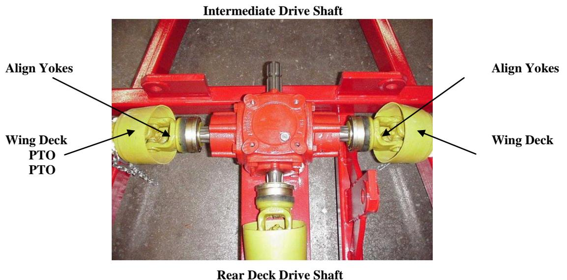
All PTO shafts have a short chain attached on both ends. Find a location to
